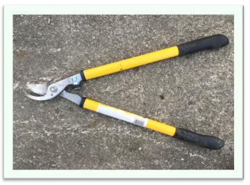
The lopping shears are for the thicker in width branches and are used to prune branches from a half inch to an inch in diameter.
