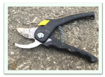
The pruning shears are for the smallest width branches and may prune branches up to a half inch in diameter.
