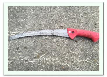
The pruning saw is for any branches thicker than an inch diameter.
